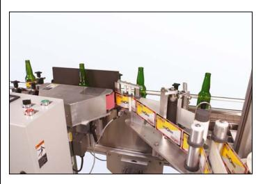
length can be reconfigured, along with the direction of the machine (left-hand vs. right-hand) and one of three labeling styles — wrap, spin-in-place, or trunnion style. So changing your line layout or the packages you run does not make the labeler you already purchased obsolete.
